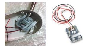
Fig 8: Typical 3 Wire Strain gauge 3.4 Microcontroller System Wiring Diagram Here we have the microcontroller system implementation wiring diagram. The display units are connected at port 1, set input at port 2 and finally the display drivers at port 0. 3.5 Output Display Interface Wiring Diagram The 7 – Segments displays are interfaced at port 1 of the microcontroller. Four displays are multiplexed and driven with four transistors. A single display is shown figure 12.
